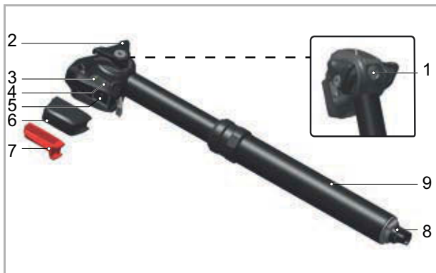
Figur 39: Opbygning ROCKSHOX Reverb AXS sadelpind
